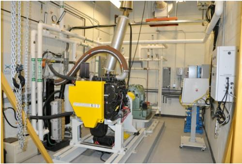
*Among the facilities of Golisano Institute for Sustainability (GIS) is a dedicated laboratory for internal combustion research. The Engine Dynamometer Laboratory is staffed and equipped for investigations of engine performance and emissions resulting from use of biofuels formulated in a variety of blends.*
