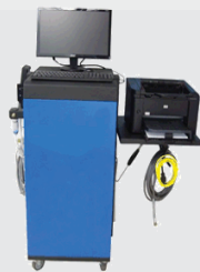
5 Gas Analyzer System
