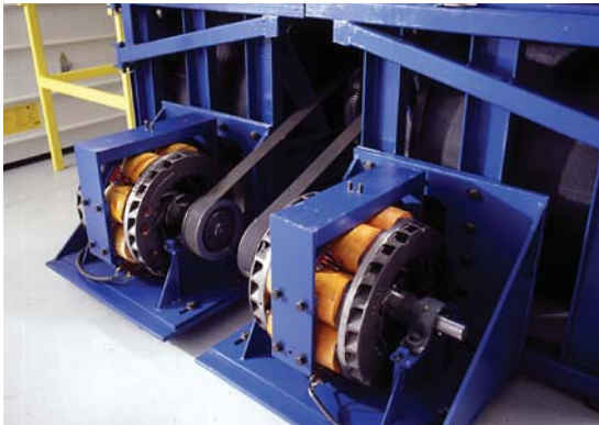
A look at Mustang's Dual Eddy Current PAUs - photo shows dynamometer with PAU cover removed
