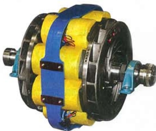
The eddy-current power absorption unit uses electromagnetic voltage (controlled by a computer) to generate the braking torque at the rollers required to allow steady state and controlled acceleration runs.
