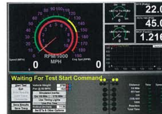
Mustang's PowerDyne software provides a wealth of information to the operator and provides clear and simple controls for unique features like its quarter-mile drag race simulation.
