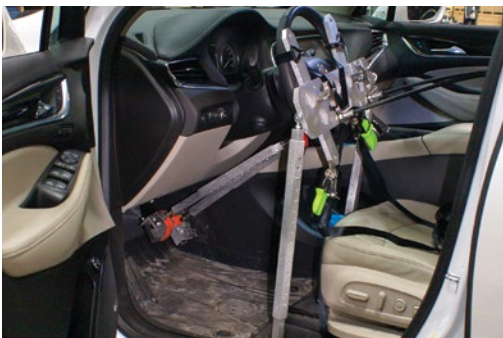
Robotic pedal-throttle actuators for automatic driving
